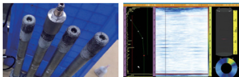
Wind Turbine Bolt Inspection(Cylindrical Guided Wave)
