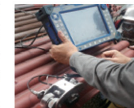
Corrosion Inspection of Boiler Water Wall
